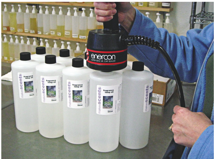
Makes Scents founder Joanne Klauber uses an induction sealer, left, to help prevent leaks from filled bottles during shipment. A table-top, air-pillow maker, right, saves valuable shop floor space with its small footprint and just-in-time manufacturing capabilities.
