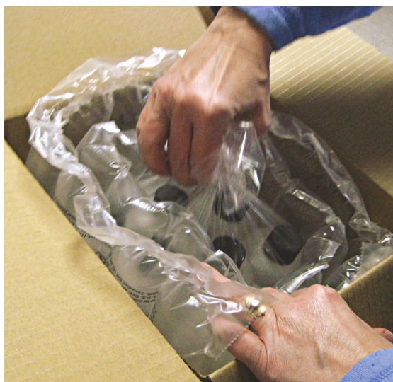
In addition to being a more space-efficient alternative, air pillows offer better protection for Makes Scents' bottled lamp oils.
