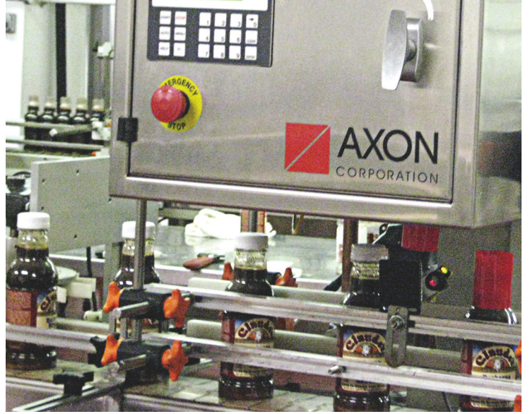
A labeling system applies wraparound UV-coated paper labels to the bottles, left. The labeling system is equipped with two stepper-driven label applicators. The bottles then travel to a tamper-evident bander that applies neck bands that go over the edges of the caps and extend down to the shoulders of the longneck bottles.
