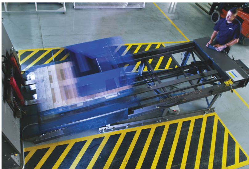
Moving pallets from an end-aisle stand, the SRM automatically stores and retrieves pallets from the rack system.
