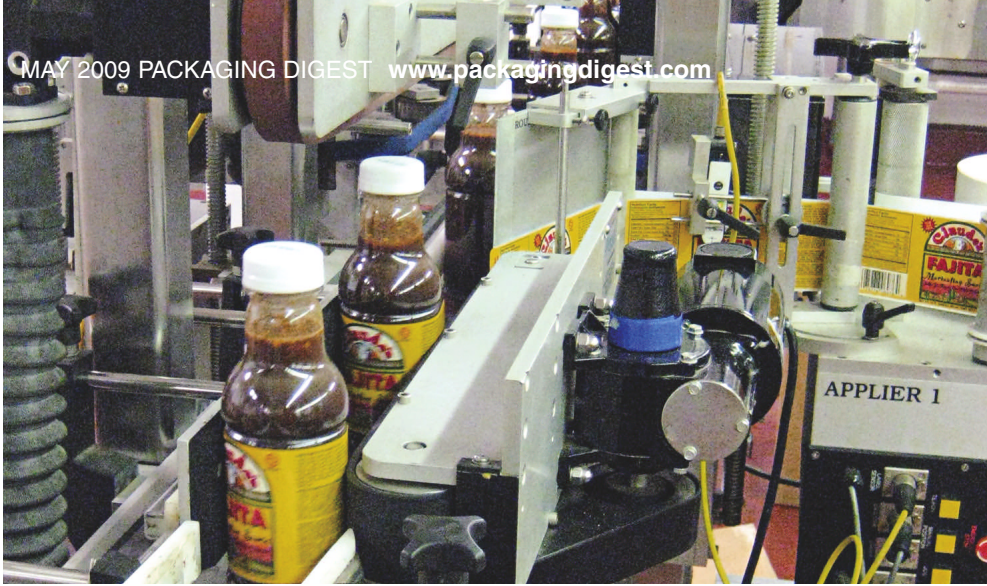
A labeling system applies wraparound UV-coated paper labels to the bottles, left. The labeling system is equipped with two stepper-driven label applicators. The bottles then travel to a tamper-evident bander that applies neck bands that go over the edges of the caps and extend down to the shoulders of the longneck bottles.
