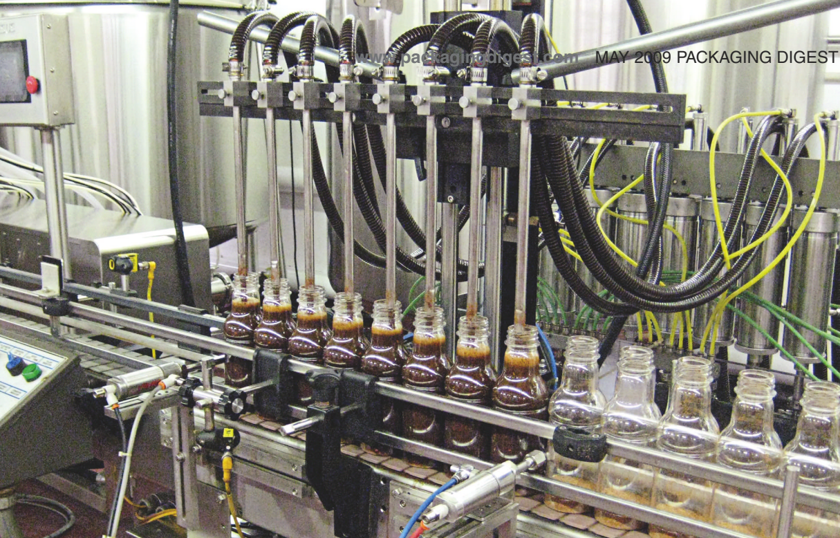
Liquid components are filled on an intermittent-motion, in-line filler that fills eight bottles at a time.
