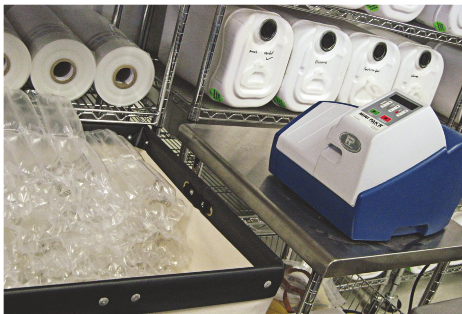
Makes Scents founder Joanne Klauber uses an induction sealer, left, to help prevent leaks from filled bottles during shipment. A table-top, air-pillow maker, right, saves valuable shop floor space with its small footprint and just-in-time manufacturing capabilities.
